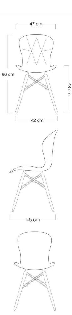
Total Weight: 4.5 Kg with high quality wood lumbers with Grade AA, cross made of iron with a thickness of 7 mm and polyethylene coating also retaining joints between the wood and the floor of the chair made of iron belt with a thickness of 3 mm.
